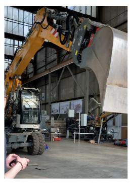
What opportunities do 5G networks offer for heavy machinery? You can discuss the answer to this question with the developers, while controlling an 18 t wheeled excavator with a game controller via 5G Campus network with low latency. Control signals as well as sensor variables for real-time visualization are provided interoperably via OPC UA — an industry driven standard for every type of machine.
